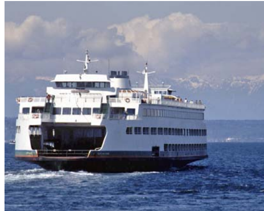
Photo 1: WSDOT operates the nation's largest ferry system – the Spokane carries up to 188 vehicles and 2000 passengers in the Puget Sound and San Juan Islands.
