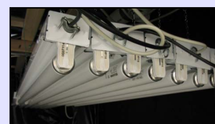
Figure 3. Ambient light treatment + UV (LL + UV). Four Sylvania F40 T12 CWP bulbs plus three Q-Panel Corp UVA-340 bulbs
