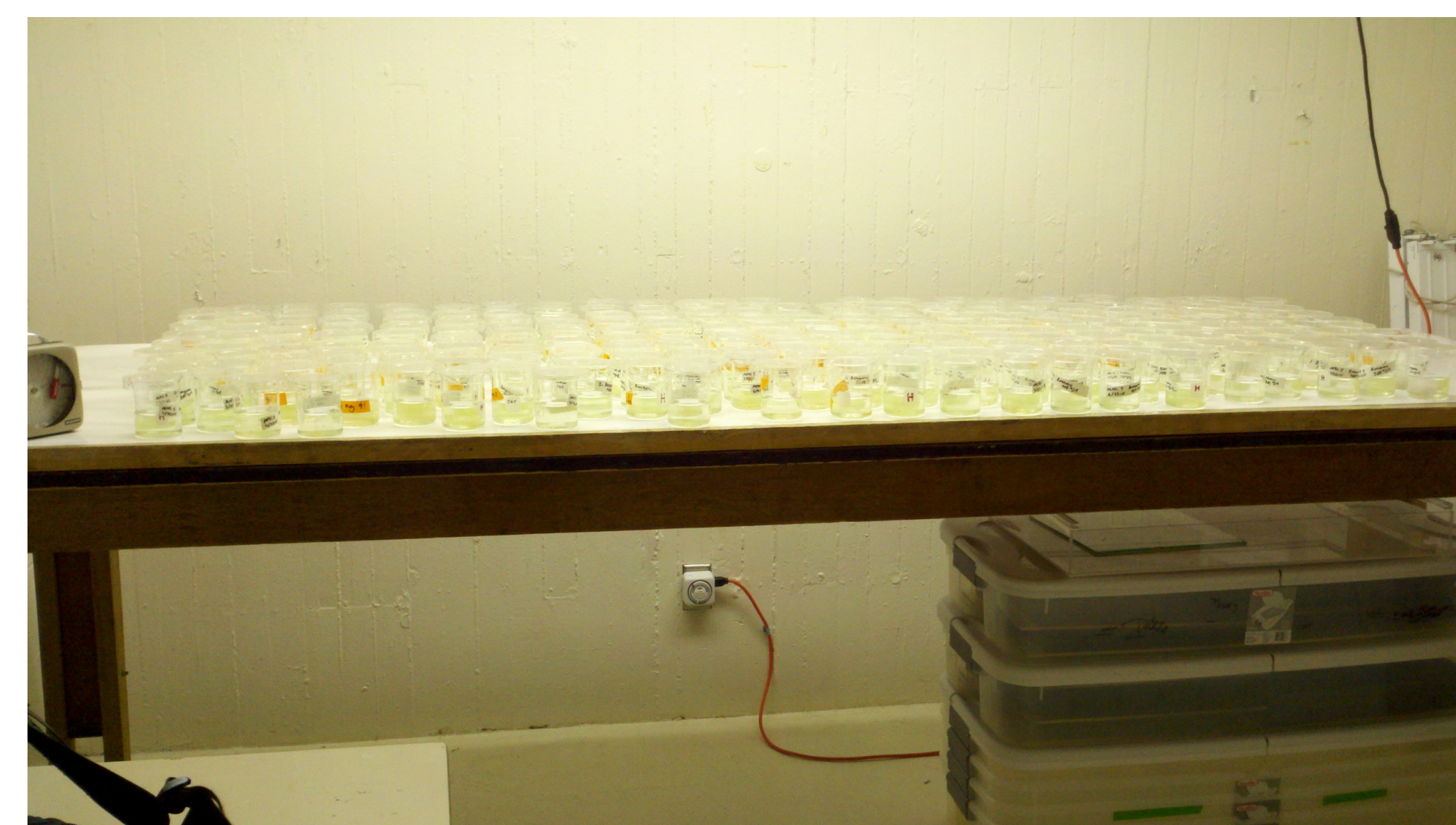
Figure 1. Set up of malathion, benzene, mixture, and negative control test chamber beakers on day one of exposure, February 23 rd , 2011.
