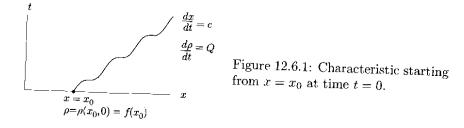
**Example.** If the local wave velocity c is a constant  $c_0$  and Q = 0, then the quasi-linear partial differential equation (12.6.1) becomes the linear one, (12.2.6), which arises in the analysis of the wave equation. In this example, the characteristics may be obtained by directly integrating (12.6.3) without using (12.6.2). Each
