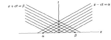
Figure 12.3.1: Characteristics for the one-dimensional wave equation.
