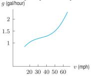
Figure 4.37: Gas consumption versus velocity
