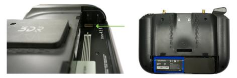
Figure 7.1.6.1: Controller Battery Installation
