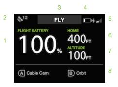
Figure 4.5.2.1: Controller In-Flight Data Display
