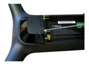
Figure 7.5.1.1: GPS Cover Removal
