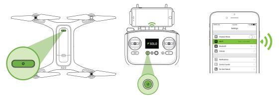
Figure 2.6.2.1: Connect to Solo Link
