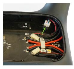
Figure 7.4.3.1: Compass Connector on Mainboard
