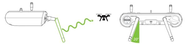
Figure 3.11.5.1: Controller Antenna Orientation
