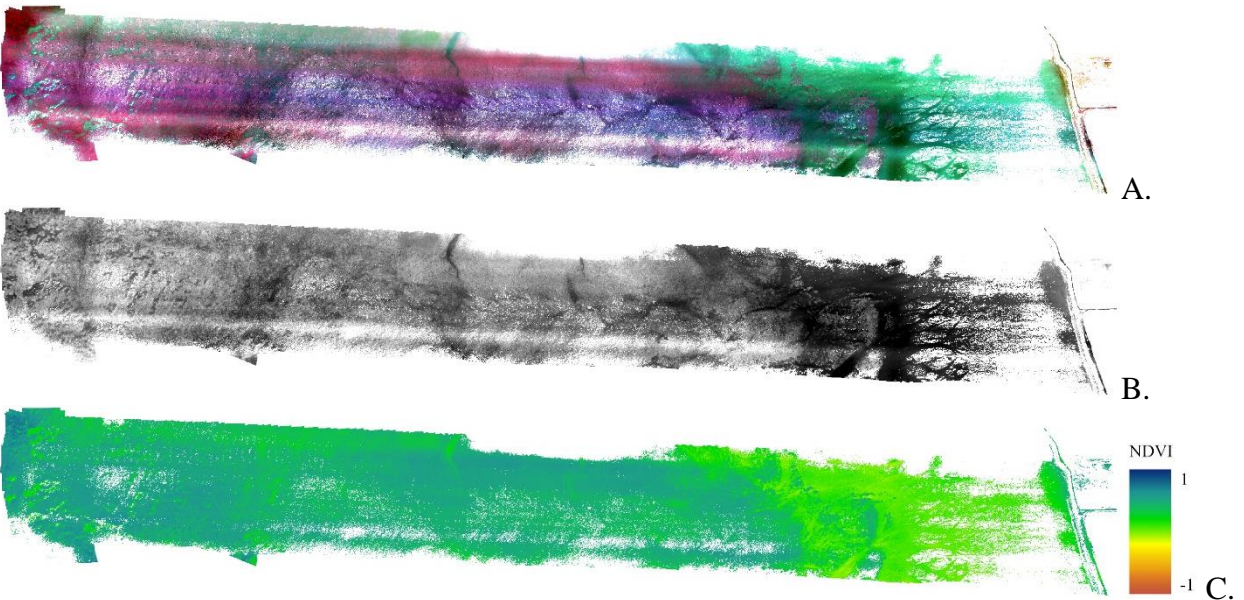
Figure 15. Orthomosaics created from imagery collected on June 23, 2020 in A) color infrared (bands 10, 6, 4), B) infrared (band 10), and C) NDVI.
